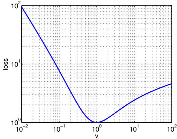
**Fig. 7.** NLPD loss (up to a constant) incurred when predicting at a single point with a Gaussian predictive distribution. In the figure we have fixed  $\|t_i - m_i\|^2 = 1$  and show how the loss evolves as we vary the predictive variance  $v_i$ . The optimal value of the predictive variance is equal to the actual squared error given the predictive mean.
