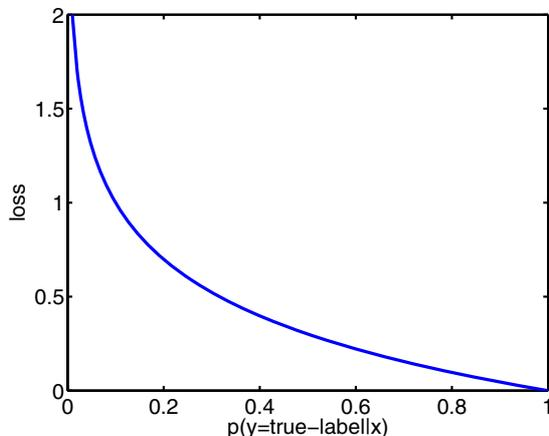
**Fig. 5.** NLP loss when predicting the class of a single test point that actually belongs to class “+1”. Observe how the loss goes to infinity as the model becomes increasingly certain that the point belongs to the wrong class.
